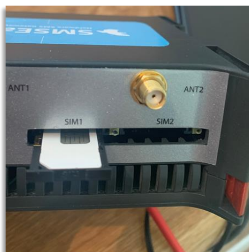
Figure 110: Inserting the SIM card and SIM tray into the SMSEagle
