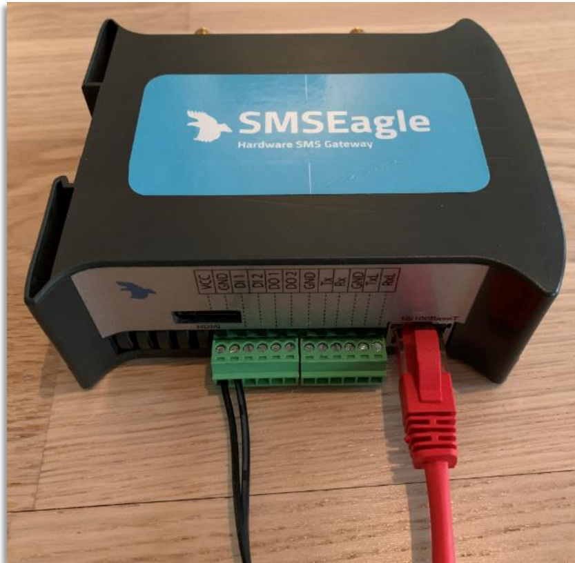
Figure 102: SMSEagle with the necessary cables connected correctly
